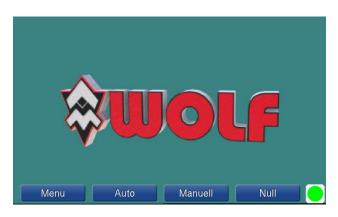
As long as no measurement data is available, the logo is displayed in the background. If measurement data is available, the last measurement value and the statistical values of the last measurement series are displayed. Operation display (bottom-right) shows the current status of the measuring device. (Green -> ready for a measuring task / Red -> measuring device is in an active measurement)
