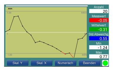
The automatic measurement is started immediately. A submenu with *Scal. Y / Scal. X / Numeric / Exit* controls the graphical display or is used to stop the measurement.
