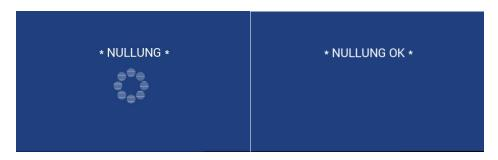
The measuring sensor moves at a speed of 2.5mm/sec to the measuring table and remains there for 2 s until the measuring sensor is set to "0.000" at this point.
