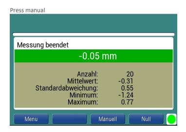
This is the access point for manual measurement. The individual measurement is triggered with Start (or by pressing the foot-operated switch). The display is graphical and numerical. The scaling works as described for the automatic measurement. To return to the main menu, press "Exit".
