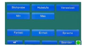
**Sample** = number of measuring points to be measured (with automatic measurement)
